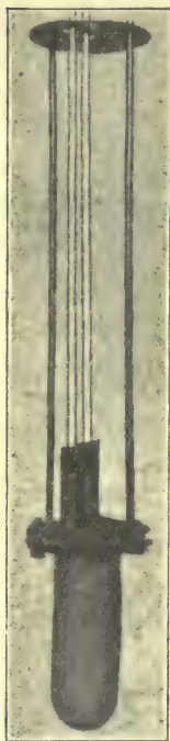
FIG. 52.—Osmometer of W. Billz and A. von Vegesack.
